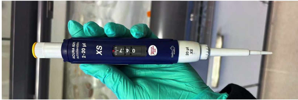
Figure 8. Detailed view of the micropipette used for single-cell isolation.
